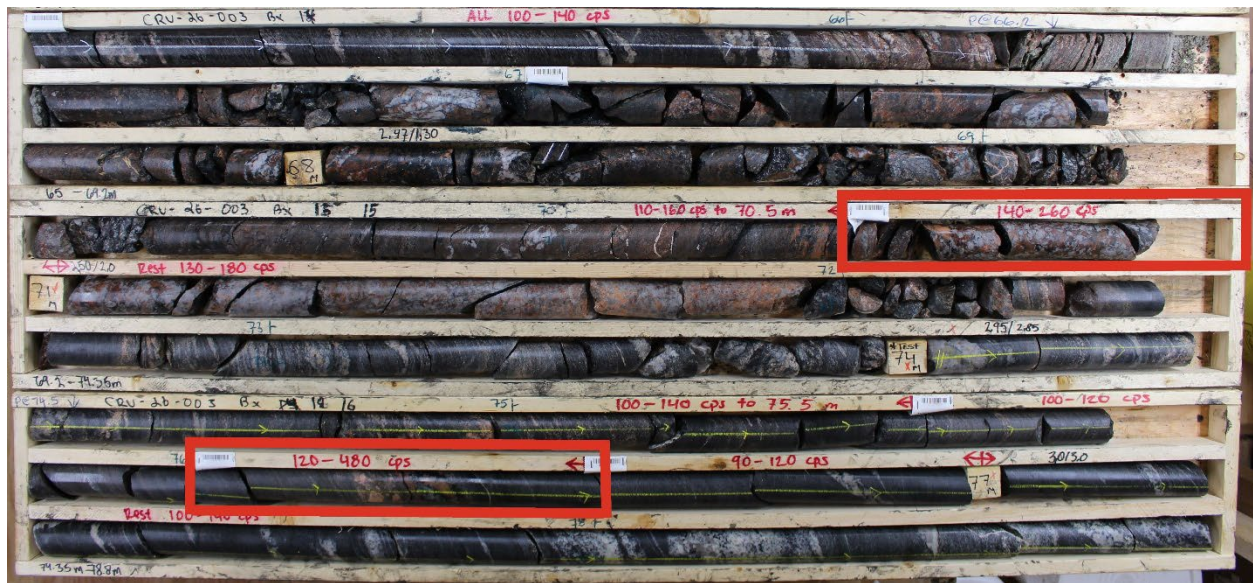
Figure 4. Drill core photos from CRV-26-003 highlighting anomalous uranium associated with hydrothermal alteration and structure. Geochemical assay of a fractured and hematized zone returned 64.4 ppm partial uranium over 0.5 m from 70.5 to 71.0 m. From 76.0 to 76.5 m, semi-pelitic gneiss with local pegmatite intrusion returned 76.2 ppm partial uranium (0.008 wt.% U_3O_8 ) over 0.5 m.
