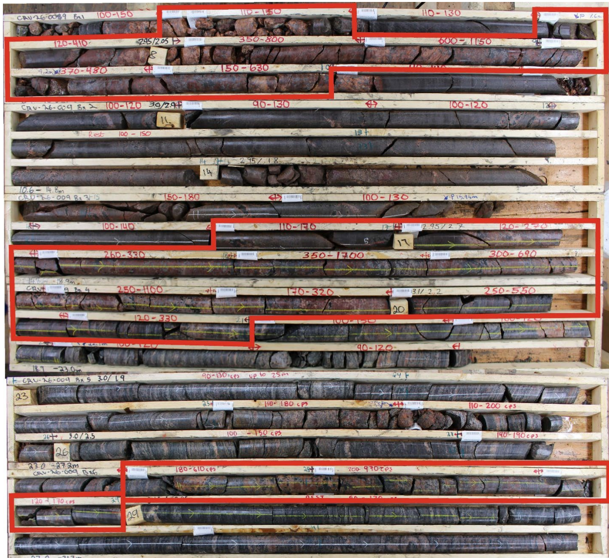
Figure 8. Drill core photos from CRV-29-009 highlighting anomalous uranium values associated with hydrothermal alteration and structure. Assays returned uranium values of 0.0005 wt.% to 0.018 wt.% U_3O_8 (10.1 to 192.0 U ppm, partial) over 3.0 m between 6.5 to 10.0 m; values ranging from 0.0005 up to 0.019 wt.% U_3O_8 (11.1 up to 171.0 U ppm, partial) over 4.5 m from 16.5 to 21.0 m; and values of 0.001 wt.% up to 0.035 wt.% U_3O_8 (27.0 ppm and 300 U ppm, partial) over 1.5 m from 27.5 to 29.0 m.
