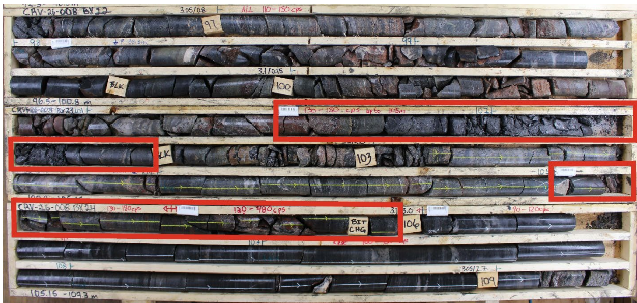
Figure 6. Drill core photos from CRV-26-008 highlighting anomalous uranium associated with hydrothermal alteration and structure. Graphitic brittle reactivated fault zone within pelitic gneiss characterized by strong to locally intense graphitic gouge hosts 21.2 ppm partial uranium over 1.0 m from 101.5 to 102.5 m. Below, geochemical assays returned 0.003 wt.% U_3O_8 (36.1 ppm, partial) over 0.5 m from 105.0 to 105.5 m and 0.024 wt.% U_3O_8 (201.0 ppm, partial) over 0.5 m from 105.5 to 106.0 m associated with hematized pelitic gneiss.
