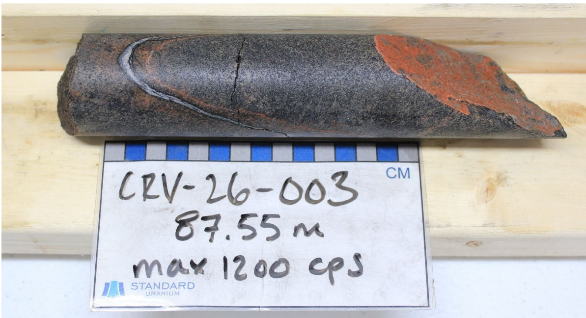
Figure 3. Drill core (NQ 47.6 mm diameter) photo from hole CRV-26-003 highlighting cross-cutting carbonate vein and associated hematite alteration hosting radioactivity up to 1,200 cps at 87.55 m.
